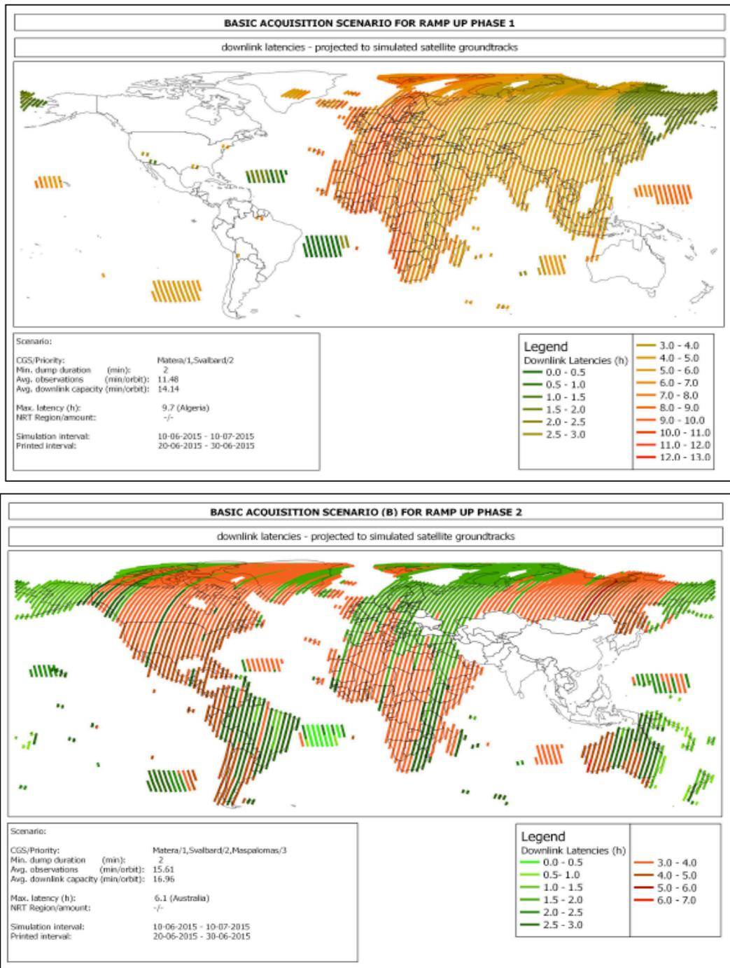
Figure 4.1 – Two-phased approach of the basic acquisition scenario during the 9 months ramp-up phase with downlink latencies projected to simulated satellite groundtracks.
