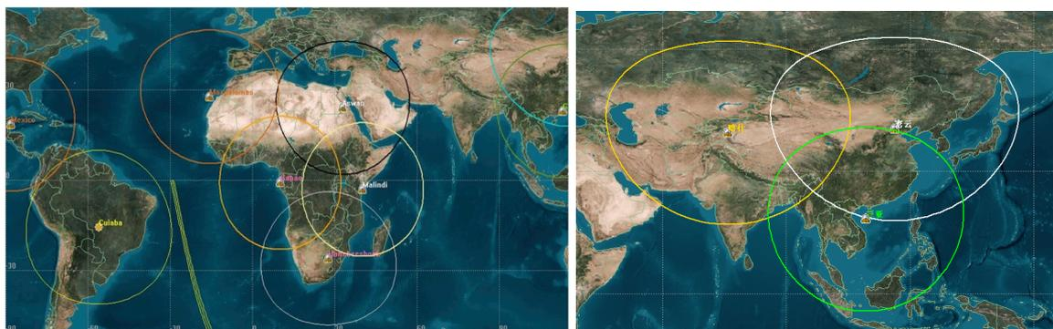
Figure 4.4 – CBERS-4 ground station coverages for INPE (left) and for CRESDA (right).
