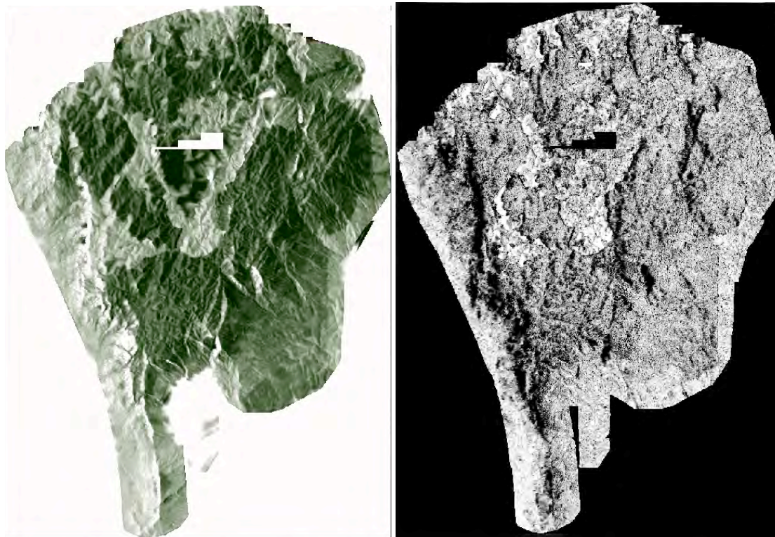
Figure 2.8.6. Tandem-X InSAR height (i.e., the height of the centre of the RADAR backscatter above ground; left) and coherence (right) obtained for Amani National Park. Logged areas can be distinguished from intact forest as the InSAR heights of the former are close to zero and the coherence is high (bright areas; right).
