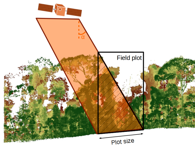
Figure 3.2 Illustration of the mismatch generated by an incidence angle ( \alpha ) of ca. 30^\circ and a field plot size of ca. 25 m. The hashed polygon illustrates the match existing between the forest volume measured by both the satellite sensor (in orange) and from the field (black). In this example, the large heterogeneity of the forest at the plot scale would result in significantly different biomass estimates from the satellite and ground measurement.
