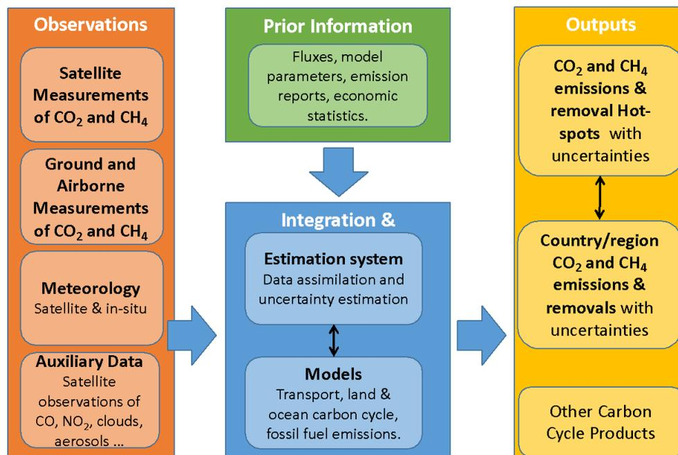
Figure 1: System functional overview an atmospheric CO<sub>2</sub> and CH<sub>4</sub> monitoring system, showing the key inputs, outputs, and interactions.
