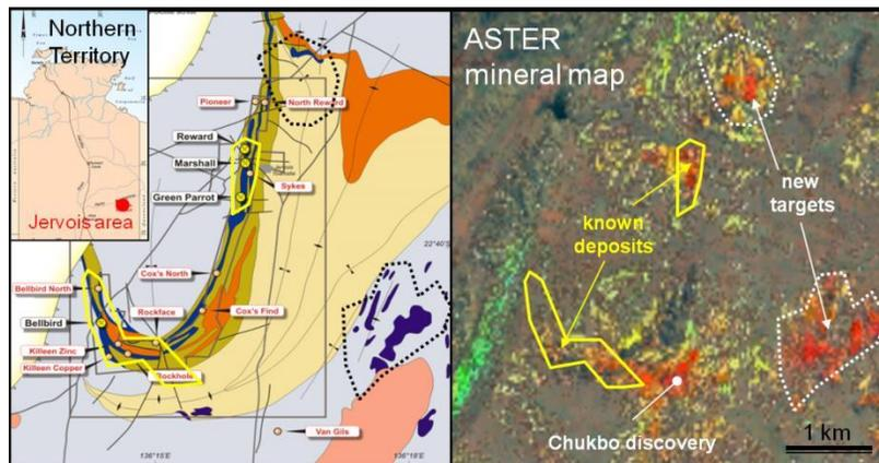
Fig 1: (left) published geology and mineral occurrences in the Jervois area, Northern Territory (from Kentor Gold); and (right) propylitic alteration (warmer colours) evident in the ASTER "MgOH" product, which was critical in the discovery of Chukbo.
