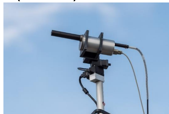
Ground-based PANDORA spectrometer Column density O_3 , NO_2 , HCHO, and SO_2
