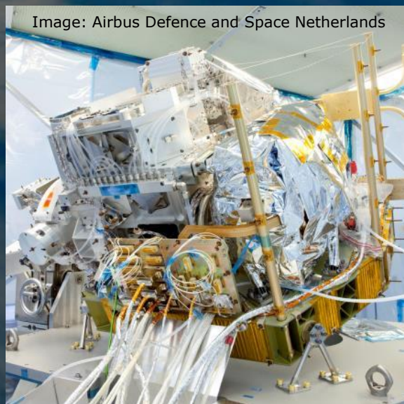
Assembled TROPOMI instrument
