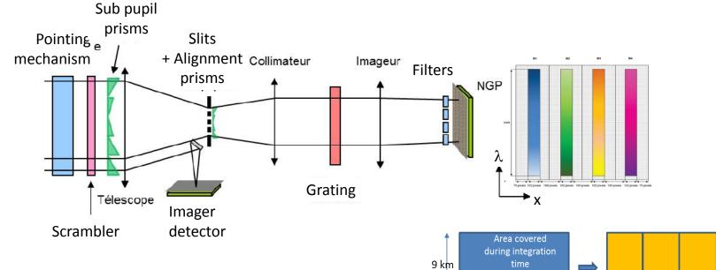
Innovative concept permitting the acquisition of the 4 spectral bands with a single telescope, spectrometer and detector (NGP Sofradir)
