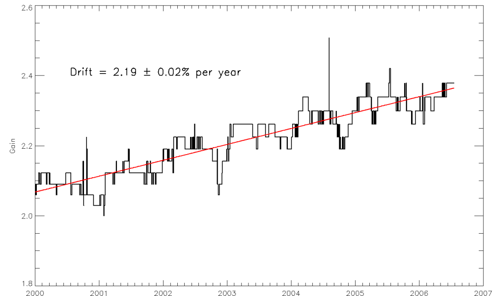
Gains for Meteosat-7/VIS using Aqua/MODIS Reference via DCCs
