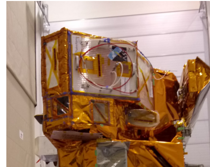
IASI FM3-R on Metop C with Cold Box radiator protection cover
