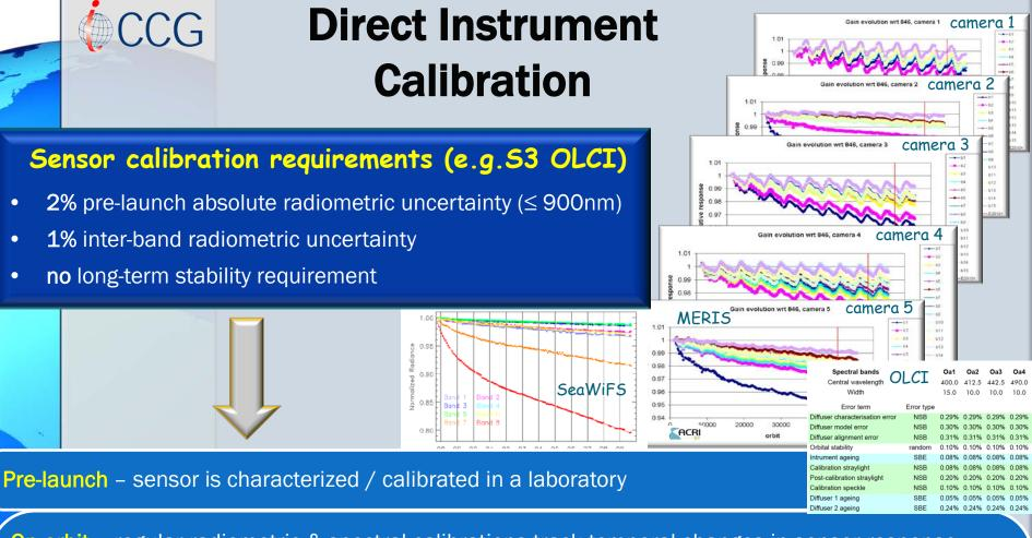
On-orbit – regular radiometric & spectral calibrations track temporal changes in sensor response
