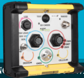
XEOS Resolute GNSS receiver (Septentrio board)
