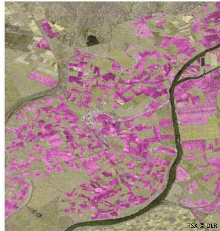
Fig.: TerraSAR-X false colour composite image (HH / VV / HH-VV) of a test site in the mouth of the Guadalquivir river, SW of Spain, acquired on August 4. Cultivated rice fields are identified in pink colour (Lopez-Sanchez et al., 2011)
