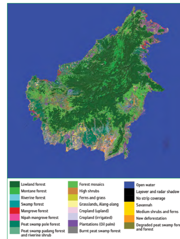
Figure 5: Wall-to-wall land cover map over Borneo island derived from ALOS PALSAR data Credit: D. Hoekman, Wageningen UR, NL
