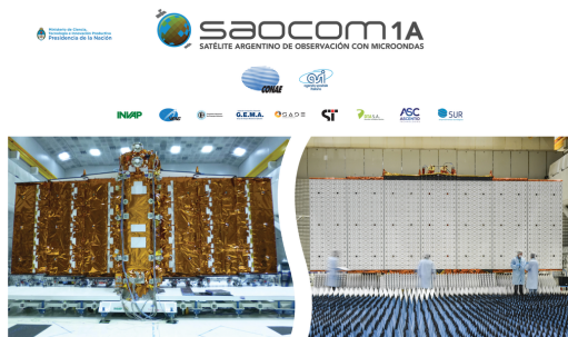
Figure 5: The SAOCOM platform and its 35m 2 L-band SAR polarimetric antenna deployed.
