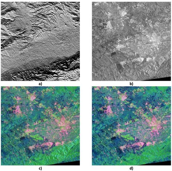
**Figure A2.1** Example of polarimetric decomposition generated from ARD covariance format. **a)** Shaded DEM of the area; **b)** RADARSAT-2 HH intensity; **c)** Yamaguchi decomposition colour composite (Red: even bounce, Green: random, Blue: odd bounce); **d)** Same as c) with terrain flattening option. Generated from Radarsat-2 FQ18W acquired over Murcia, Spain on 18 June 2014 ©MDA 2014
