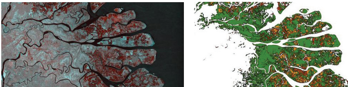
Figure 5: An example of GMW data for the Kahan River Delta, North Kalimantan, Indonesia. [Left] Multi-temporal radar image composite (1996 JERS-1 SAR and 2016 ALOS-2 PALSAR-2); [Right] Global Mangrove Watch extent and change map; Red – mangrove loss 1996-2007; Orange – loss 2007-2016; Green – mangrove cover in 2016 (Satellite image copyright JAXA/METI).
