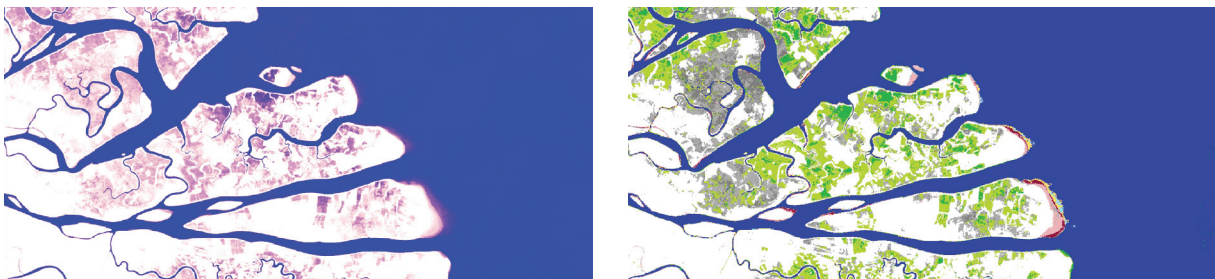
Figure 4: An example of GSWE data for the Kahan River Delta, North Kalimantan, Indonesia. [Left] Surface Water Occurrence shows where surface water occurred between 1984 and 2015 and provides information concerning overall water dynamics; [Right] Transitions map provides information on the change in surface water seasonality between 1984 and 2015 and captures changes between the three classes of not water, seasonal water and permanent water. Source: EC JRC/Google.
