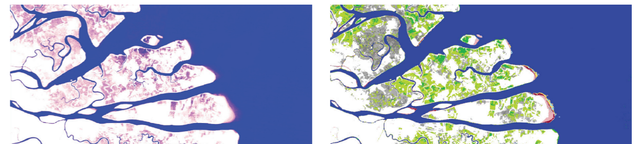
Figure 4: An example of GSWE data for the Kahan River Delta, North Kalimantan, Indonesia. [Left] Surface Water Occurrence shows where surface water occurred between 1984 and 2015 and provides information concerning overall water dynamics; [Right] Transitions map provides information on the change in surface water seasonality between 1984 and 2015 and captures changes between the three classes of not water, seasonal water and permanent water. Source: EC JRC/Google.
