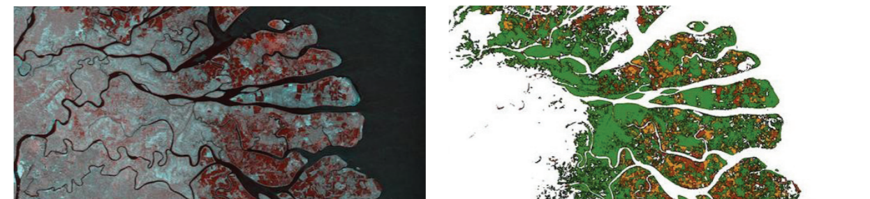
Figure 5: An example of GMW data for the Kahan River Delta, North Kalimantan, Indonesia. [Left] Multi-temporal radar image composite (1996 JERS-1 SAR and 2016 ALOS-2 PALSAR-2); [Right] Global Mangrove Watch extent and change map; Red – mangrove loss 1996-2007; Orange – loss 2007-2016; Green – mangrove cover in 2016 (Satellite image copyright JAXA/METI).
