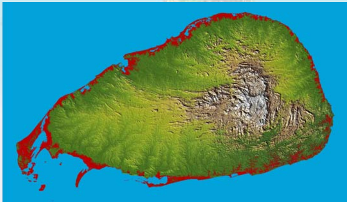
30m height “flood-fill” based on SRTM-DTED1® 3” (≈90m)
