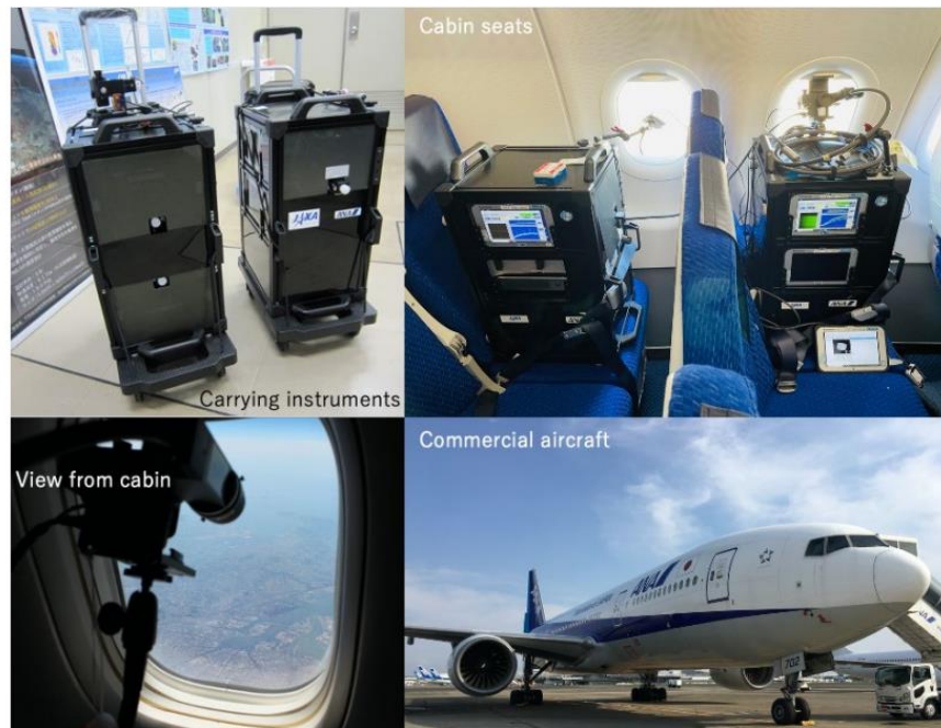
Figure 2. The GOBLEU remote sensing equipment onboard an ANA passenger aircraft.
