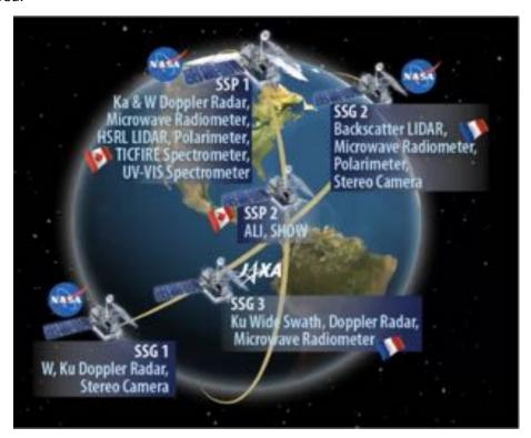
The white paper calls for a non-sun synchronous cross-calibration satellite for the precipitation constellation.
