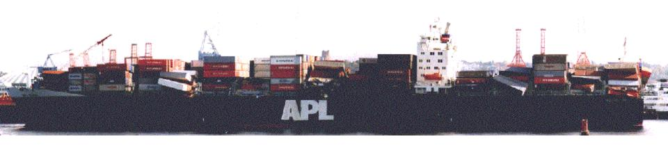
APL's M/V APL China, as it arrived in Seattle 1 Nov 1998 in the wake of Typhoon Babs. APL China lost 406 containers, with over 1,000 damaged. Similar damages were sustained by Maersk, Evergreen and other lines in Taiwan waters. Sources at APL estimated that losses were ~hundreds of millions of U.S. dollars for all vessels.
