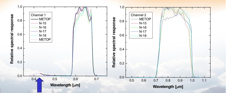
Significant spectral leak in the blue region for AVHRR/METOP ch.1.
