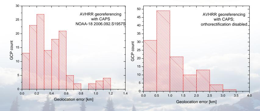
Geolocation error is calculated by comparison the reprojected AVHRR scene with MODIS reference (composite) image in LCC projection. Comparison is performed by chip matching. Here, the MODIS composite for April 01-10, 2006 was used.
