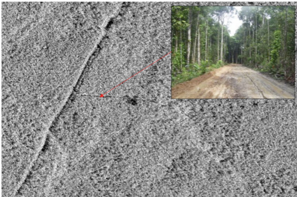
Figure 13. Guyana. Logging road detected in Very Fine Resolution (1 m) radar data. (Image credit: DLR, Photo: Hoekman/U.Wageningen)
