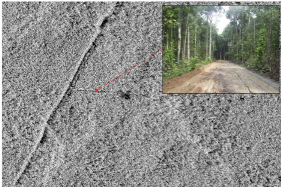
Figure 4. Guyana. Logging road detected in Very Fine Resolution (1 m) radar data. (Image credit: DLR, Photo: Hoekman/U.Wageningen)
