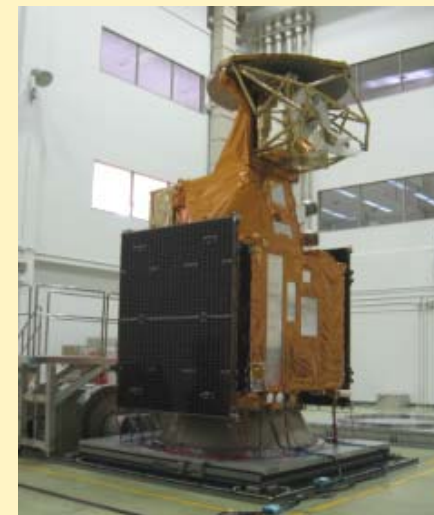
Vibration Test (January 2011)
