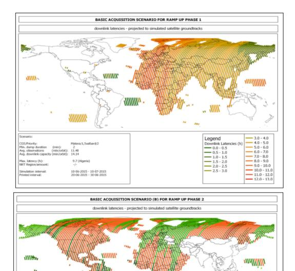
*Figure* 4.1 – *Two-phased approach of the basic acquisition scenario during the* 9 *months ramp-up phase with downlink latencies projected to simulated satellite groundtracks.*
