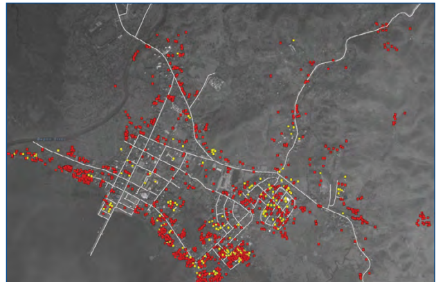
Figure 2: Satellite EO-based product using very high-resolution optical imagery (WorldView satellite) to analyze the damaged structure caused by the Super Typhoon Haiyan in November 2013. In red, the destroyed structures; in yellow, structures that may be damaged. This map was elaborated by UNITAR/UNOSAT, which regularly collaborates with the Charter. The same methodology is also very useful to estimate damage after an earthquake.
