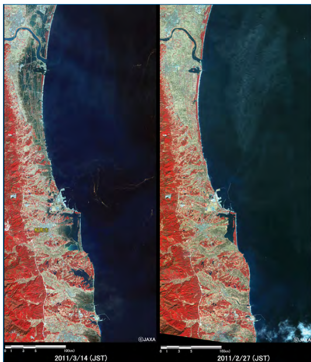
Figure 4: These images from JAXA's ALOS radar satellite were taken before (right) and after (left) the Great East Japan Earthquake and subsequent Tsunami. Areas flooded by water appear dark blue in the post-disaster image.
