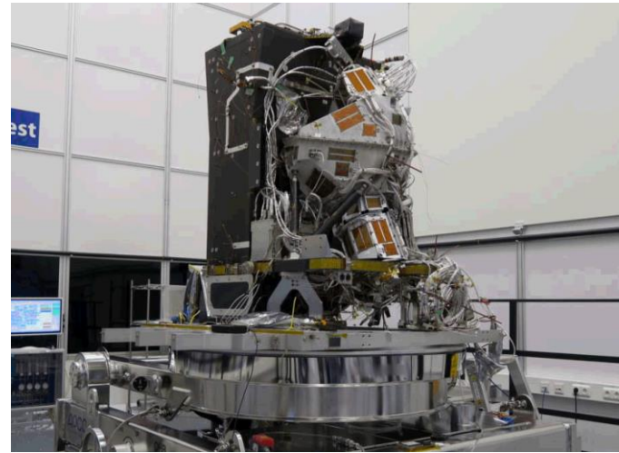
PFM Optical system integrated and aligned into the Instrument Module; Airbus Courtesy
