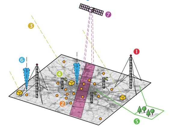
Tall towers (1), street level mid-cost sensors (2), roof level stations (3), eddy covariance flux stations (4), ecosystem parameters (5), total column GHG and meteorology (6) and satellite (7) observations, in many parts including co-emitted species (from: ICOS Cities)
