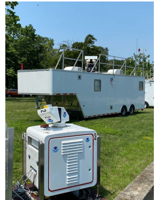
NOAA Doppler lidar and TOPAZ O 3 lidar trailer at YCFS (photo: A. Langford)
