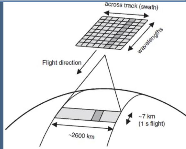
CrIS ground track illustration taken from Han et al., 2013. MUSES algorithm allows FOV thinning to reduce processing overheads.
