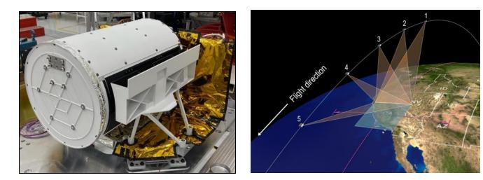
The instrument contains a 14-band spectro-polarimetric camera that is pointable in two axes:
