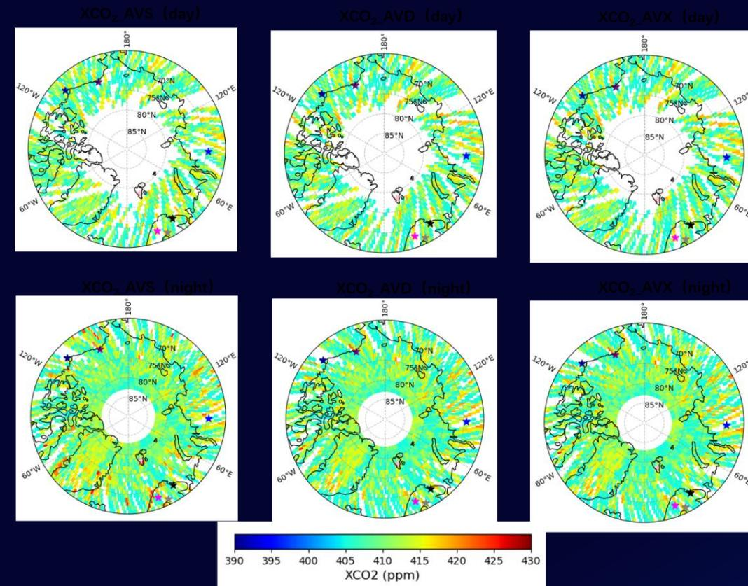
Compared with passive detection, active carbon dioxide lidar can detect surface reflectance at high latitudes and high altitudes such as polar regions, as well as carbon dioxide at night.
