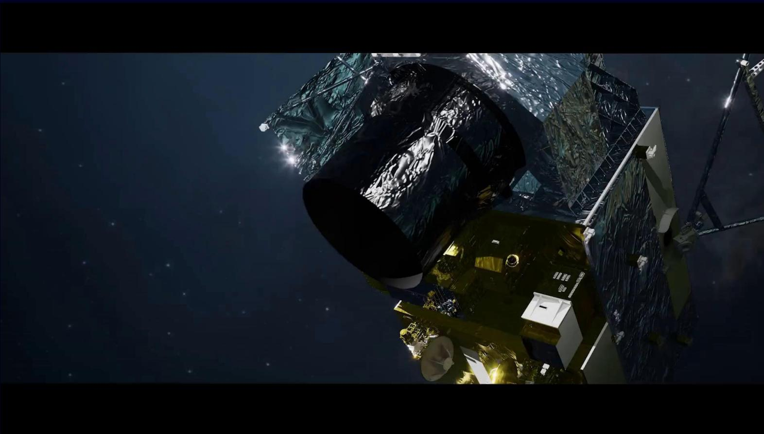
DQ1 is equipped with the world's first active LiDAR carbon dioxide instrument, simultaneously emitting two laser beams, located on the absorption and non absorption lines respectively
