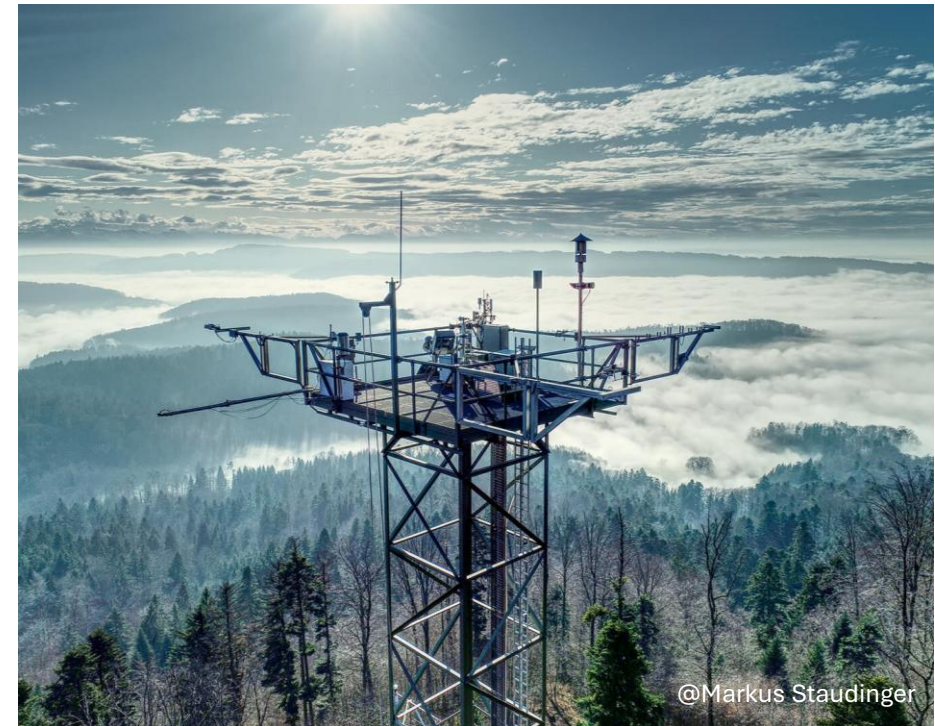
AmeriFlux / ICOS flux towers — point measurement ( ~1 km footprint, TROPOMI collocation \pm 2 h) .
