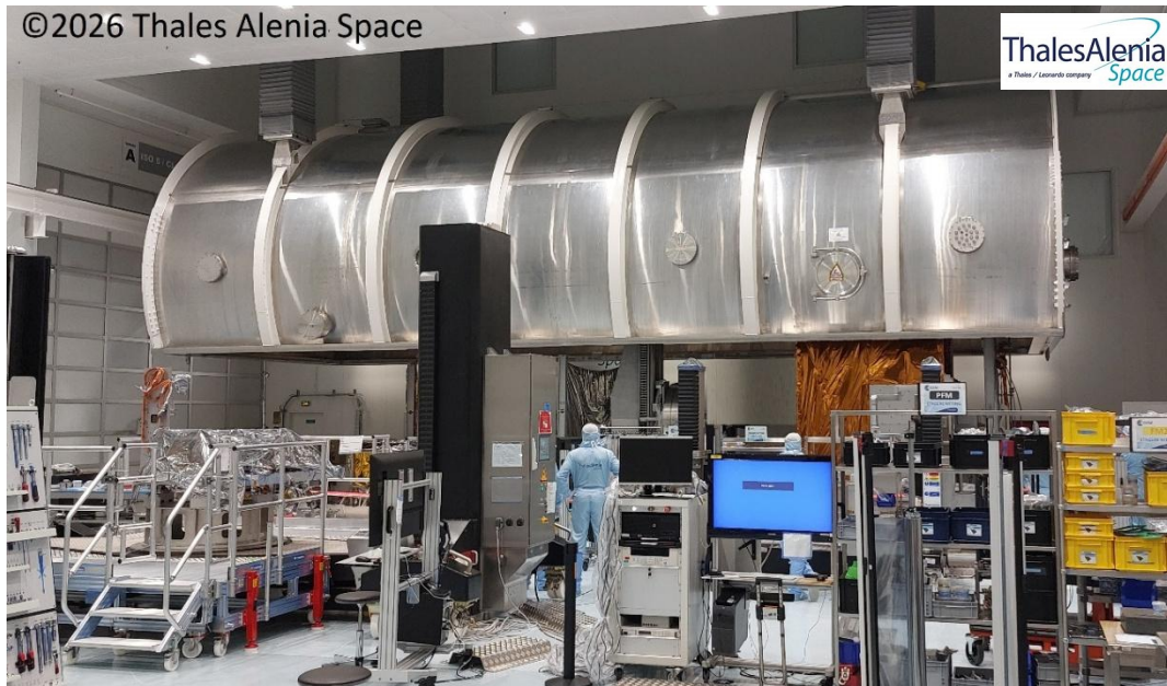
Vacuum chamber closure for CO 2 I determination of alignment
