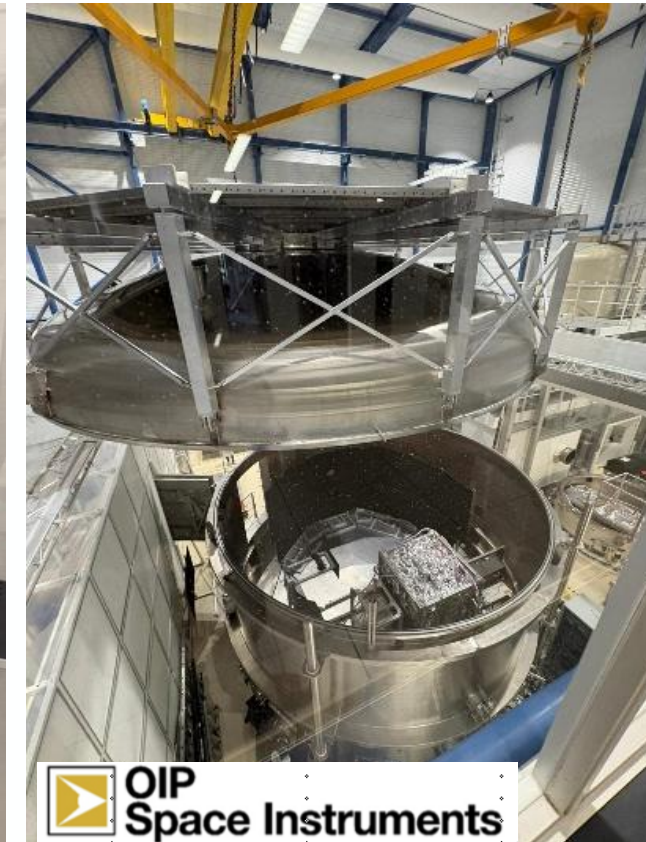
CLIM PFM in CSL facility for characterisation and calibration
