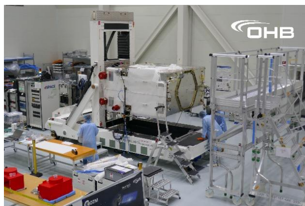
Platform subsystems Electrical Power (EPS) Solar Array: 3 panel wing steered by SADM Battery Li-ion with 3 modules AOCS Gyroless architecture, 3-axis stabilized satellite Safe mode based on magnetorque/magnetometer Propulsion and Reaction control (RCS) Mono-propellant in blow down with 8 Thrusters (20N) 2 Propellant Tanks with 250 kg capacity TT&C S-band system providing TM/TC and ranging Data Handling Central on-board Computer and 3 Remote Terminal Units Data Storage Mass Memory 3.8 Tbits (EoL) Data Downlink Ka-band system with ka-band steering antenna and VCM (variable coding and modulation) Single channel (1.8 Gbit/s) Format Interface to Ground PUS-C, File Based Operations/CFDP Re-entry Controlled re-entry as baseline Compatible with in-orbit satellite removal
