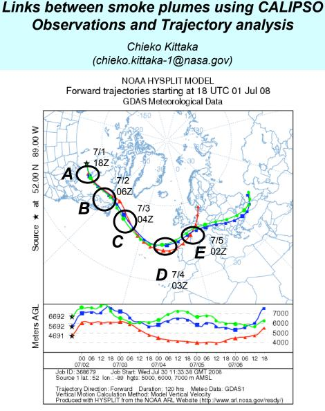
CALIPSO observations and trajectory analysis suggest that the **smoke plume A** was transported across N. Atlantic Ocean at altitudes between 5 km and 7 km and reached W. Europe on 7/4 (**plume D**). It continued moving eastward (**plume E** on 7/5).
