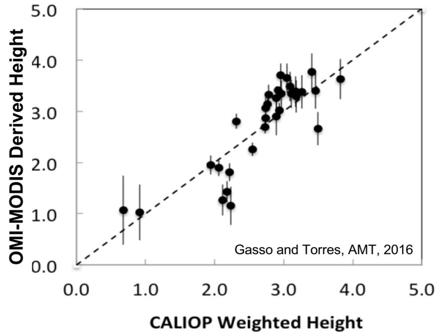
Comparison of retrieved aerosol layer height to lidar observations
