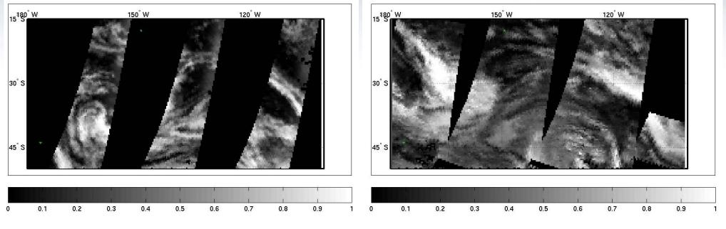
960 km swath, 24 across pixel, ~40x40 km2 Total coverage: 2 days Metop-A/B 1920 km swath, 24 across pixel, ~40x80 km2 Total coverage: 2 days Metop-A 1 day Metop-A/B
