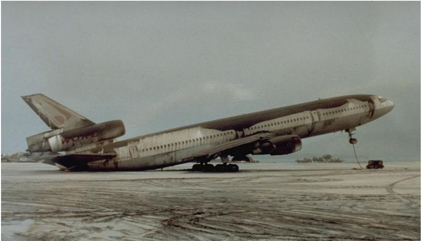
World Airways DC-10 after ash plume encounter - 1991 Pinatubo eruption
