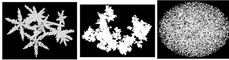
Figure 6.4. Three particle models representing an ice particle with the same dimensions and mass. Left panel - aggregate. Middle panel - fractal particle. Right panel – “soft-spheroid”. The figure is adopted from Tyynelä et al. (2011).
