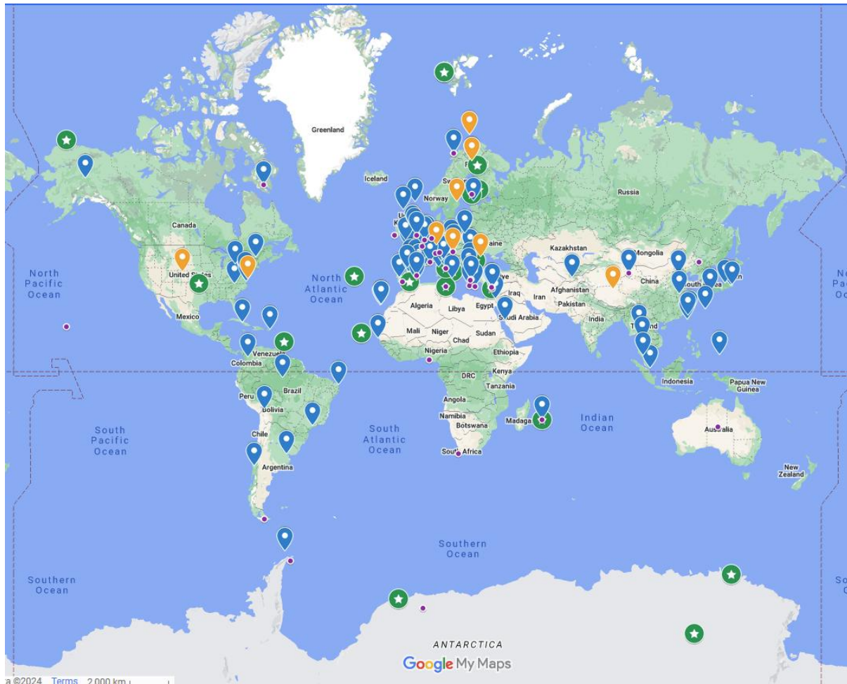
Figure 9.1. Continuously updating map with respect to EarthCARE validation stations on ground. Blue: High power lidar stations, Orange: Cloud radar stations, Green: Synergistic lidar+radar stations. Purple: Other validation measurements. Map shown at: https://www.google.com/maps/d/viewer?mid=1u1BfCIB7Sh4g5HkHqhIMO18LcDjP1MrY&usp=sharing
