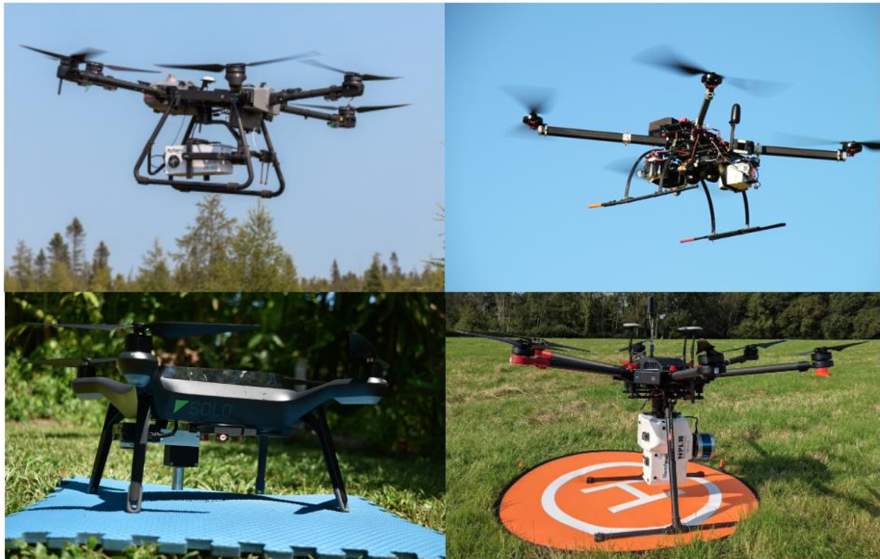
Figure 6. Clockwise for top left: Low Altitude Advanced Hyperspectral System (LAHYS) developed by NRC and the Applied Remote Sensing Laboratory at McGill University, which features a HySpex pushbroom imager (image credit: Juan Pablo Arroyo-Mora; Arroyo-Mora et al., (2023)); Rikola 2D frame hyperspectral imager from the National Land Survey, Finland (image credit: Eija Honkavaara); Ocean Optics STS point spectrometer from Maitec (image credit: Stefan Maier); Headwall Co-aligned pushbroom imaging spectrometer at NPL (image credit: Rosalinda Morrone).
