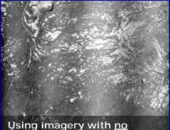
Using imagery with <u>no</u> antenna pattern compensation
