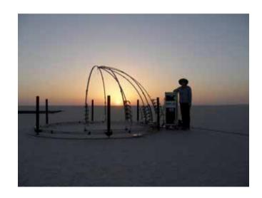
NPL Gonio-Radiometric Absolute Spectrometer System (GRASS), measurements of both surface BRDF, but also angular sky radiance.
