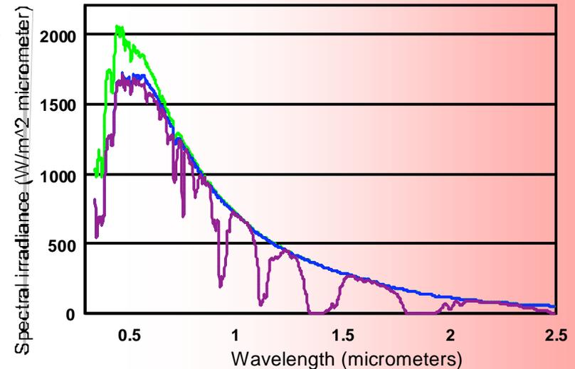
Model-based atmospheric transmittance versus wavelength
