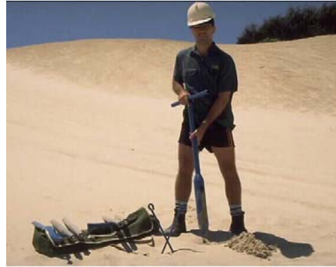
Sand auger sampling wind blown beach sand. Ocean is behind the dune.
