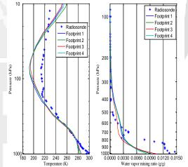
Surface temperature and atmospheric profiles retrieved from hyperspectral thermal infrared data
