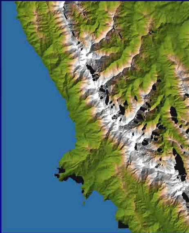
SRTM Voids & Water Mask Errors
