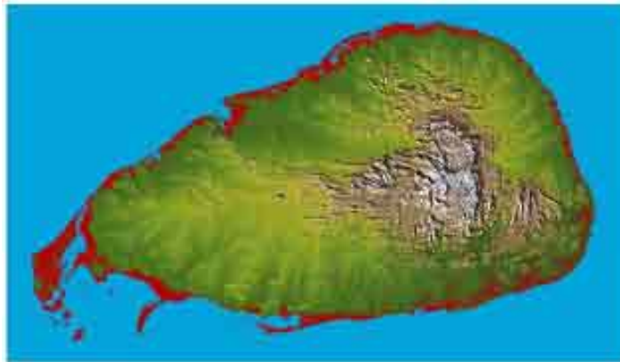
30m height “flood-fill” based on SRTM-DTED1® 3” (≈90m)
