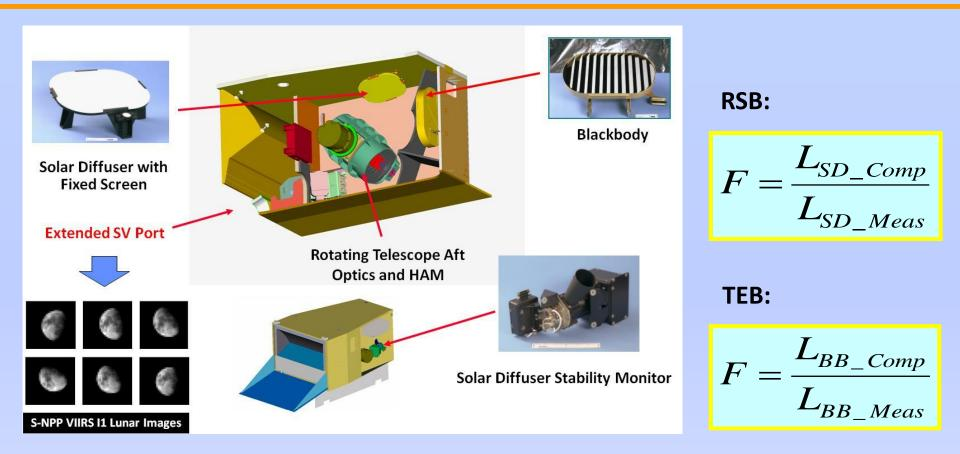
Quadratic calibration algorithm for both TEB and RSB Linear calibration coefficients derived from BB and SD SD degradation tracked by SDSM Lunar observations
