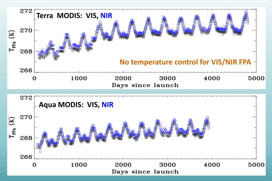
**VIS & NIR FPA temperatures: similar to instrument temperatures**
