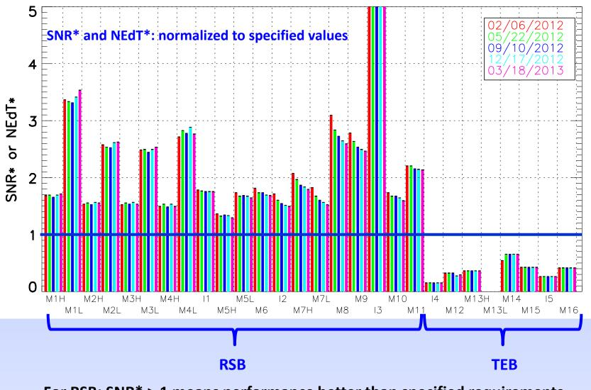
For RSB: SNR\* > 1 means performance better than specified requirements For TEB: NEdT\* < 1 means performance better than specified requirements
