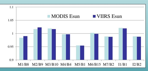
VIIRS to MODIS radiance ratios determined using sensor RSR and Esun models for their spectrally matched bands
