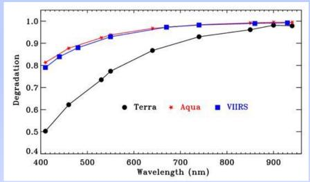
VIIRS has no SD door: Large degradation in SD BRF at short wavelengths
