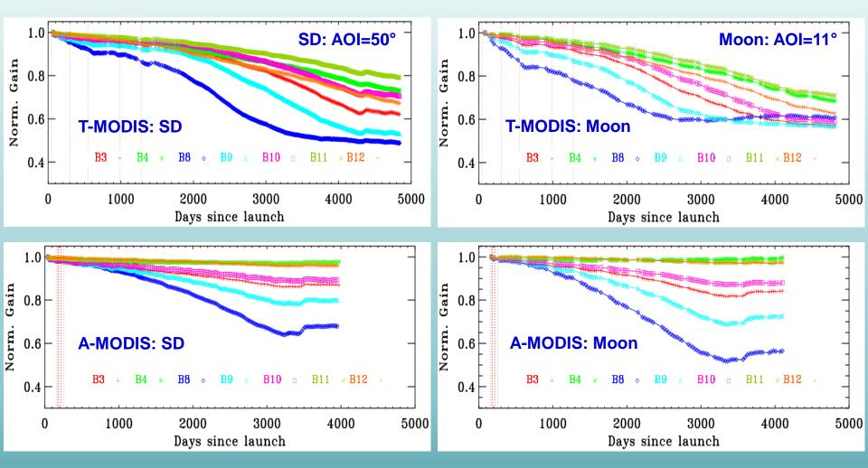
Larger changes at shorter wavelengths Wavelength, AOI, and mirror side dependent (small MS diff. in A-MODIS)
