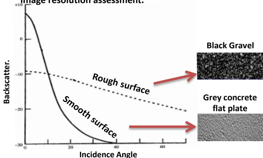
3. The size of the gravel was calculated based on both Rayleigh roughness criterion and Oh surface radar backscattering model, in order to exhibit sufficient contrast in Ku to S band radar image.
